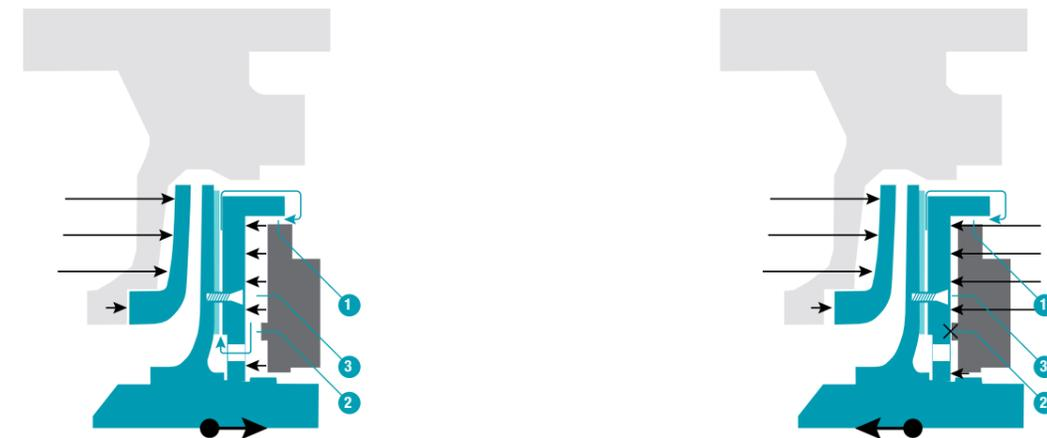
In the real functioning position, pressure in the chamber is regulated between high and low pressure. Resultant force is null and the mobile is stable and perfectly balanced between both.
