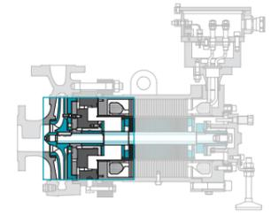
Over the years OPTIMEX has developed a performing and reliable thrust balancing system. BL+2 system is composed of two restrictions, one is stable (1), the other one is variable (2). These orifices regulate the pressure into the regulating chamber (3) that insures thrust balance of the complete mobile.
